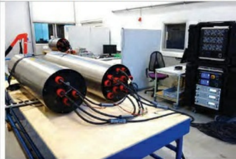
Image 18: Series 416 Li-Ion battery 430V 70kWh for 55kW manned vehicles
