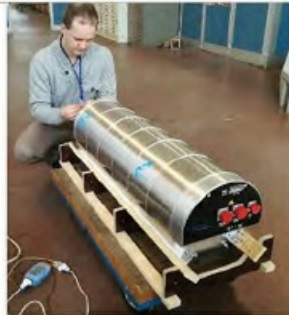
Image 17: Example of 310mm AUV battery with 6 SPB modules during installation
