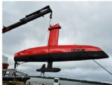
Example of a custom-made gondola (including GAPS USBL)
