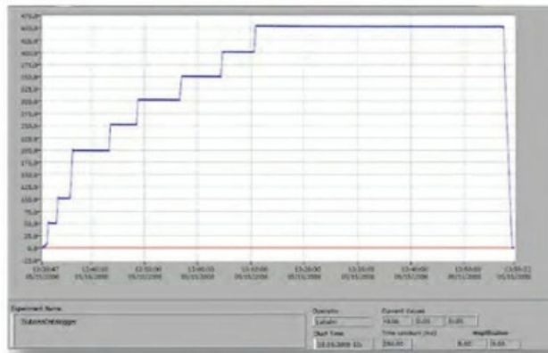
Image 38: Example test of a 4000m housing with 450 Bar test pressure.
