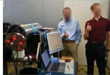
Image 14: Example of AUV battery in 6000m housing during FAT
