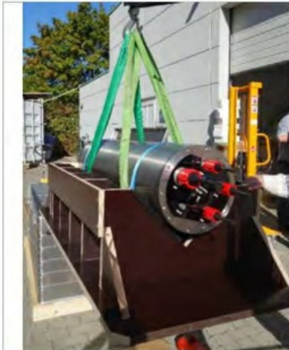
Image 33: Example of large subsea battery: 3000m
