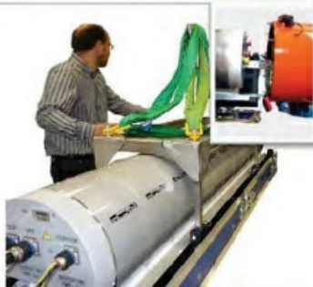
Image 15: Example of 310mm AUV battery during installation (41kWh)
